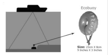
Often, marker buoys are attached to the line of underwater equipment, but these can break free and become lost. A GPS device will get you within 60 m, but with Ecobuoy attached, sonar can be used to find the equipment. When the big stationary fish symbol appears below the boat on the sonar screen, the lost equipment is directly below. By attaching a second Ecobuoy to a grappling hook, equipment retrieval is simple and easy.
